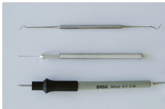
Figure 1: Instruments for tear mending: Weston dental probe (top), insect pin (centre) and hot needle (bottom)
