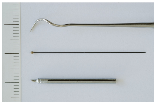
Figure 2: Tips of Weston dental probe (top), insect pin (centre) and hot needle (bottom)
