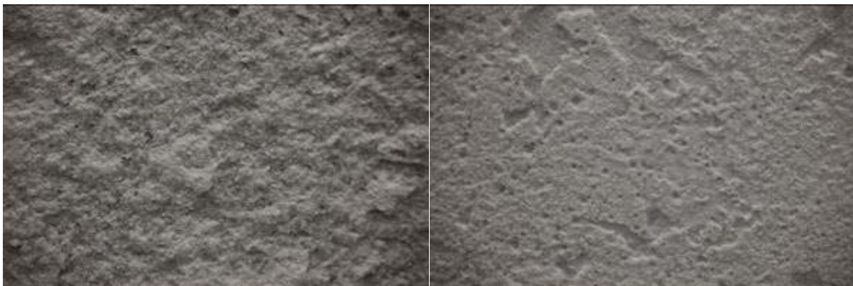
Figure 6: Failed surface at 25 minutes (left) and 25 hours (right).
