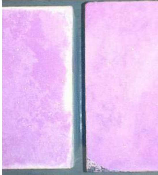
Figure 7: Phenolphthalein treated failure surfaces exposed by strength testing 25 hours (left) and 25 minutes (right) after adhesion. Pink areas, with higher pH, are uncarbonated.
