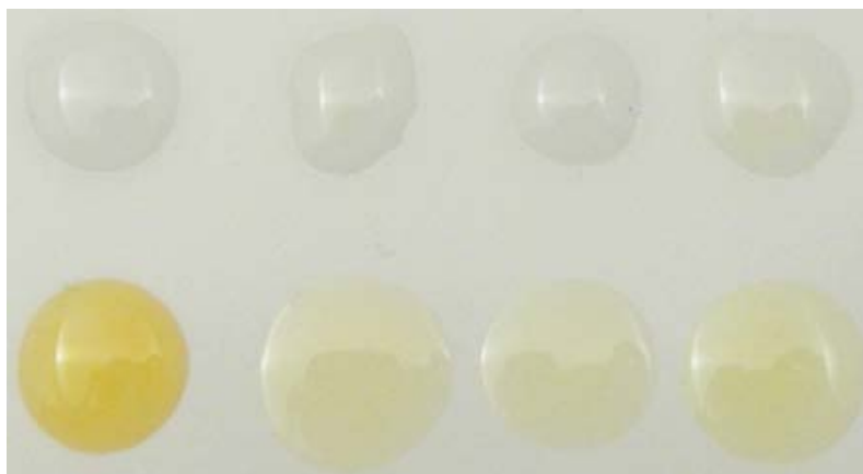
Figure 4: Part B (hardeners) before (upper row) and after (lower row) exposure to NO x . From left to right: Araldite 2020, Epo-Tek 301-2, Fynebond and HXTAL NYL-1.
