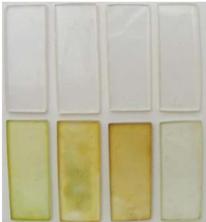
Figure 5: Epoxy adhesives test specimens before (upper row) and after (lower row) exposure to NO x . From left to right: Araldite 2020, Epo-Tek 301-2, Fynebond and HXTAL NYL-1.
