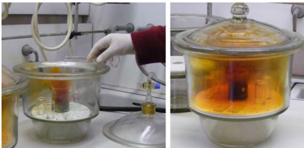
Figure 2: Production of \text{NO}_x by reaction of copper powder with nitric acid. Left: pouring of nitric acid in the beaker; right: \text{NO}_x fumes in the desiccator
