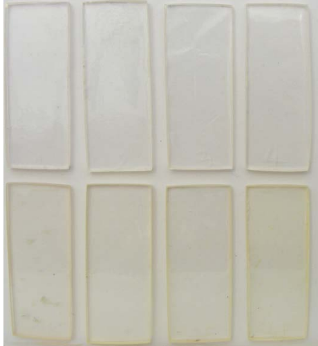
Figure 7: Test specimens before (upper row) and after (lower row) oven aging From left to right: Araldite 2020, Epo-Tek 301-2, Fynebond and HXTAL NYL-1.
