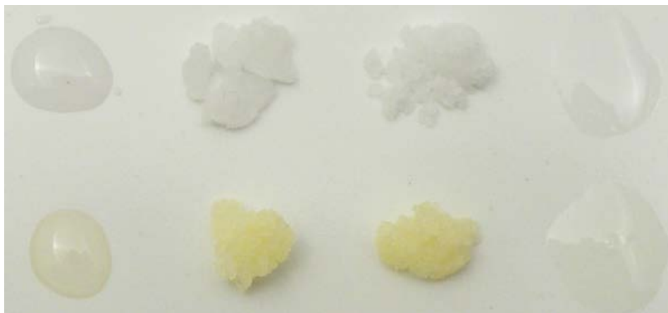
Figure 3: Part A epoxy resin before (upper row) and after (lower row) exposure to NO x . From left to right: Araldite 2020, Epo-Tek 301-2, Fynebond and HXTAL NYL-1.
