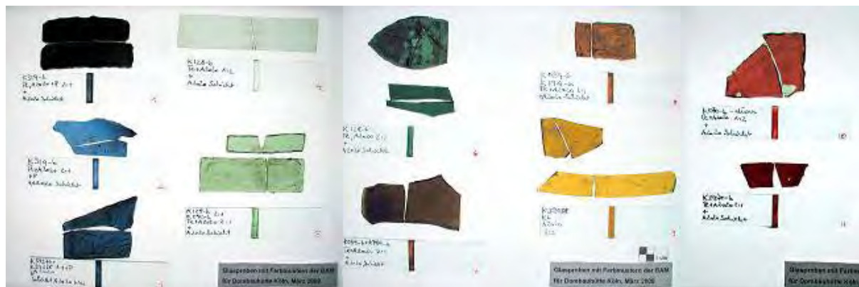
Figure 7: Samples to match the colour of medieval glass fragments, cooperation with the workshop of the Cologne Cathedral.
