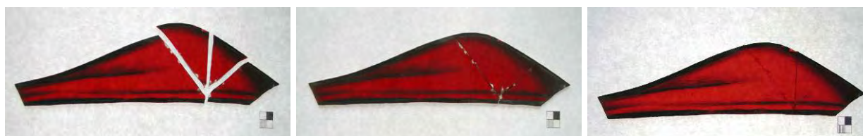
Figure 8: Broken red flashed glass (left), first work phase with transparent adhesive (middle), second work phase with adhesive-glass-powder mixture with red glass powder and red wax (right).
